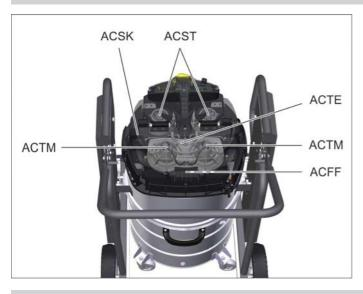
ACTM Uninstall / install Tact magnets ACSK Uninstall / install suction head ACST Uninstall/ install suction turbine ACTE Uninstall / install Tact unit ACFF Uninstall / install flat fold filter
